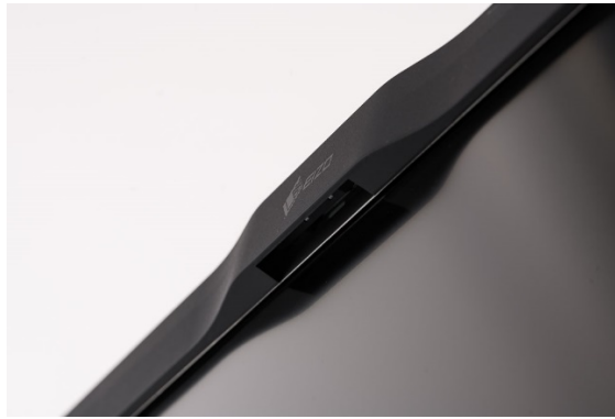
Bulge for the integrated calibration probe
